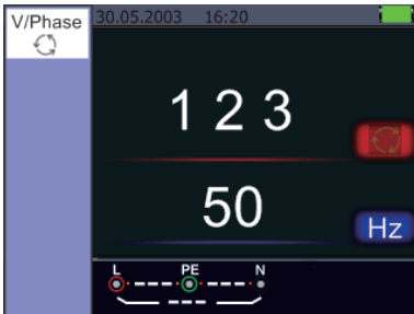
Phase Sequence Screen When connected in clockwise direction
